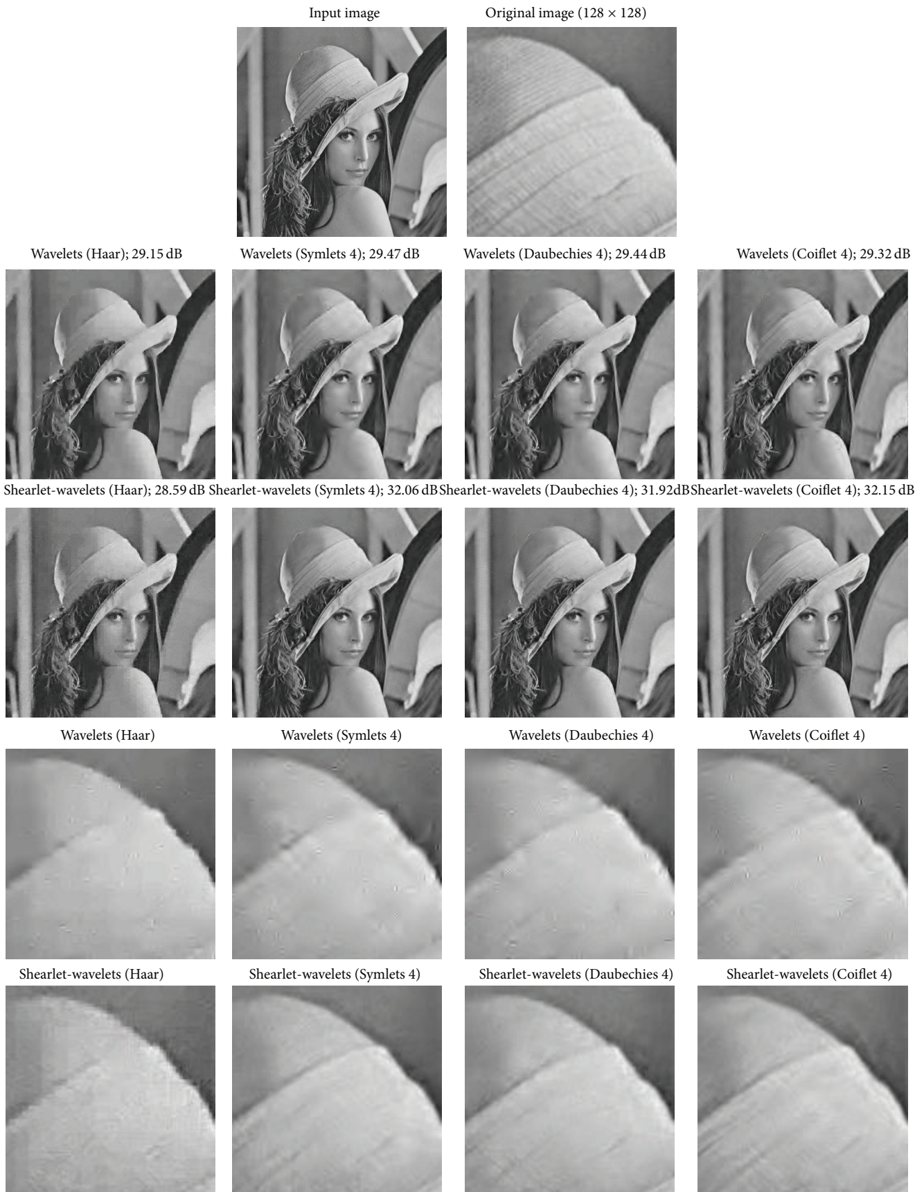
FIGURE 2: Comparison of Haar, Daubechies 4, Symlets 4, and Coiflet 4 with their corresponding combined shearlet-wavelets method.
