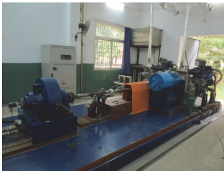
FIGURE 10: Experiment platform of hybrid propulsion shafting.
