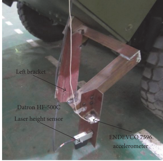
FIGURE 2: The mounted sensors of the acquisition system (left bracket).
