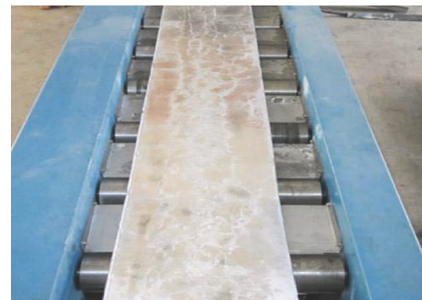
FIGURE 12: The casting 7075 aluminum alloy strip image showing the smooth surface in twin-roll strip process.
