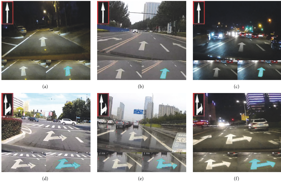
FIGURE 9: Arrow road markings recognition results: (a) recognizing Forward in nighttime; (b) recognizing Forward under cloudy condition; (c) recognizing Forward at night under lower light condition; (d) recognizing Forward-Right in sunny days; (e) recognizing Forward-Right under rainy condition; (f) recognizing Forward-Right at night.
