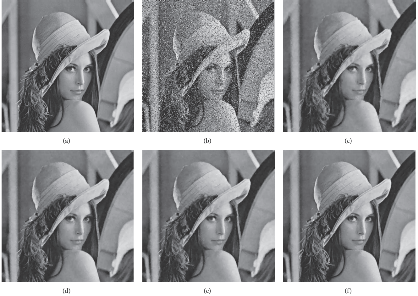
FIGURE 3: Denoising results of different methods for Lena image. (a) Noise-free image. (b) Image corrupted by mixed noise (AWGN+SPIN, \sigma=10 , p=20\% ). From (c) to (f): denoising results of TF, SBF, MNE, and the proposed algorithm.
