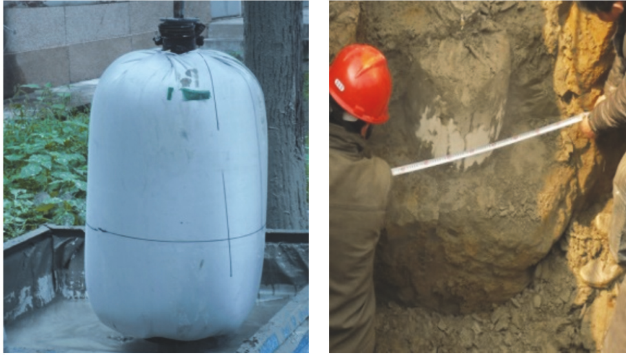
FIGURE 1: Photos of underreamed ground anchor with capsule.
