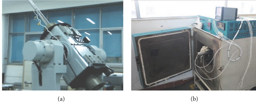
FIGURE 1: (a) Photo of the FOG error compensation experiments on the triaxial quadrature calibration bench and (b) photo of the FOG error compensation experiments in thermostat.
