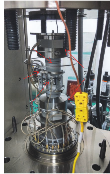
(b) Sample installation. (4) Sample. (5) Axial extensometer. (6) Radial extensometer. (7) Bearing plate and loading platform
