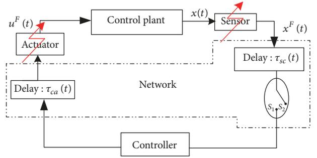
FIGURE 1: The structure of double-fault NCS.
