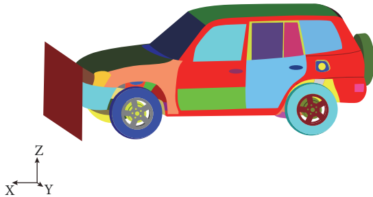
FIGURE 9: Finite element model of 100% frontal collision of minibuses.
