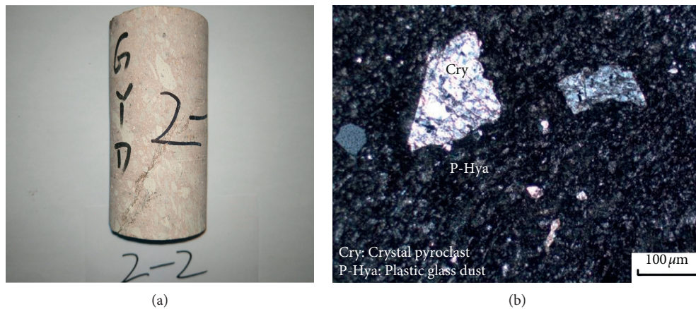
FIGURE 4: Rock type and its microscopic characteristics of the Guanyindong Slope. (a) The altered tuff samples; (b) microscopic images of the altered tuff.
