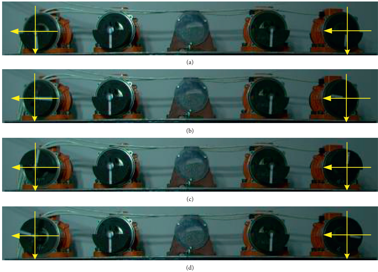
FIGURE 13: Instantaneous phase of the exciters at l = 1.3\text{ m} , n = 3 , \omega_1 = 1500\text{ r/min} , and \omega_2 = 500\text{ r/min} : (a) \varphi_1 = -7.2^\circ , \varphi_2 = 5.4^\circ , and \alpha = \varphi_1 - 3\varphi_2 = -23.4^\circ , (b) \varphi_1 = 272.8^\circ , \varphi_2 = 97.6^\circ , and \alpha = \varphi_1 - 3\varphi_2 = -20.0^\circ , (c) \varphi_1 = 189.0^\circ + 360^\circ = 549^\circ , \varphi_2 = 188.1^\circ , and \alpha = \varphi_1 - 3\varphi_2 = -15.3^\circ , and (d) \varphi_1 = 105.3^\circ + 720^\circ = 825.3^\circ , \varphi_2 = 282.1^\circ , and \alpha = \varphi_1 - 3\varphi_2 = -21.0^\circ .
