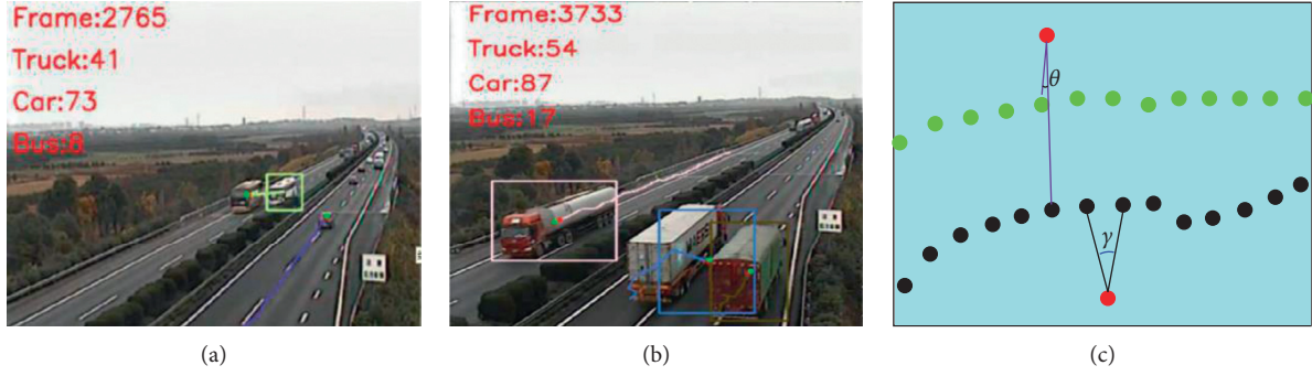
FIGURE 5: Example errors about our tracking algorithms and schematic diagram of abnormal trajectory points. We define that the forward direction is from near to far and the backward direction is from far to near. (a) The two buses occlude in the backward direction, satisfying the constraints of the tracking algorithm, but the trajectory connection is error. (b) The two trucks travelling in parallel in the forward direction also satisfy the constraints of the tracking algorithm so that the trajectory connection is wrong. (c) A schematic representation of the trajectory points of two trucks travelling in parallel for a period of time.
