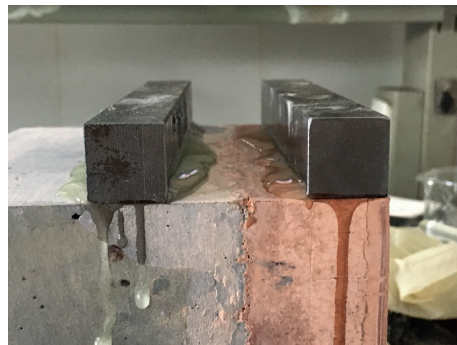
FIGURE 2: Smooth interface sample glued with two steel bar.
