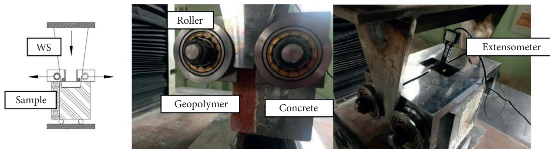
FIGURE 3: The assembled equipment for WS test.
