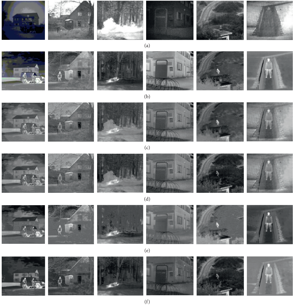
FIGURE 7: Qualitative fusion results of six images from the TNO dataset: (a) visible images; (b) infrared images; (c) DenseFuse fusion results; (d) DeepFuse fusion results; (e) FusionGAN fusion results; (f) proposed method fusion results.
