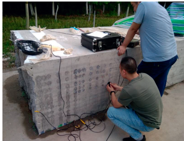
FIGURE 7: Test of P-wave velocity before and after blasting.
