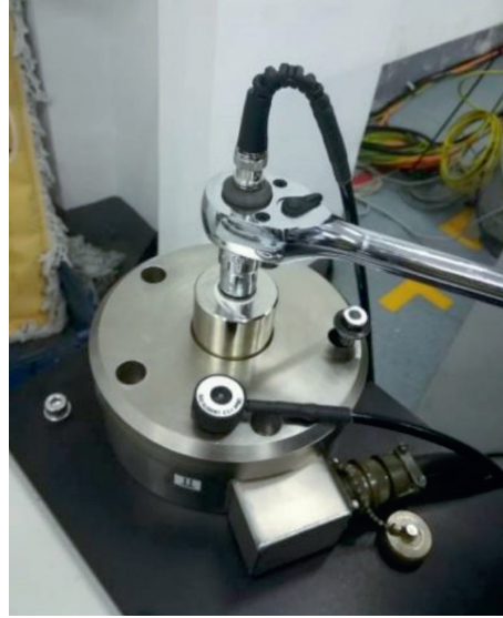
FIGURE 12: Calibration of bolt preload.
