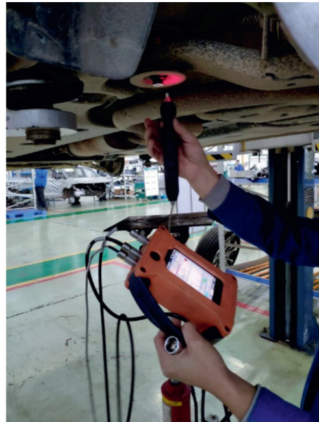
FIGURE 13: Preload measurement by the ultrasonic measuring system.
