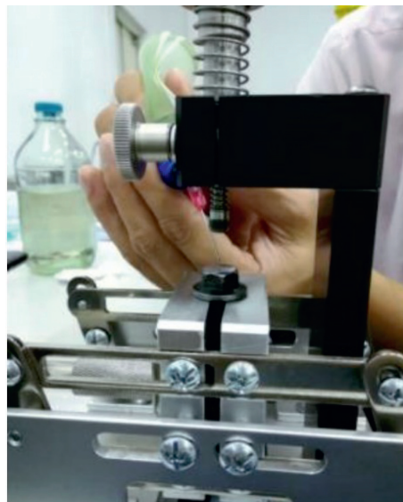
FIGURE 11: Pasting of ultrasonic transducers.
