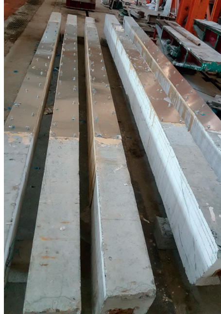
FIGURE 4: Overall appearance of strengthened beams.
