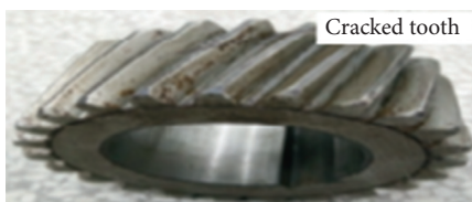
FIGURE 5: Cracked tooth fault accessories.
