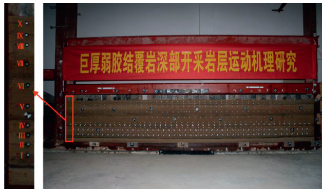
FIGURE 4: Observation lines on the similar material model.
