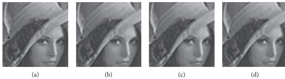
FIGURE 3: The RaSK and RaSSK algorithms for a 64 \times 64 reconstructed image. (a) is the original image, (b) is the image after sparse representation, (c) is the image obtained by the RaSK algorithm, and (d) is the image obtained by the RaSSK algorithm.
