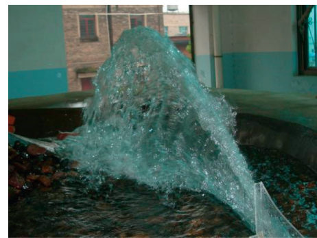
FIGURE 5: Left view of the ski-jump flow experiment in the spillway tunnel.
