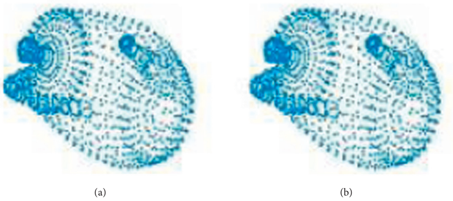
FIGURE 15: Recovered RS-coded 3D point cloud (with periodic strong pulse jamming). (a) P_w = 12.8 \mu s ( M = 0 ); (b) p_w = 51.2 \mu s ( M = 0 ).
