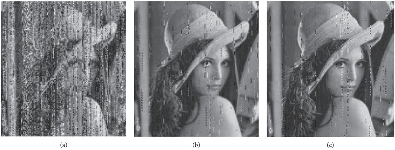
FIGURE 5: Recovered Polar-coded images (transmitted over fading channel-added periodic strong pulse jamming). (a) \text{SNR} = -2 ; \text{Psnr} = 30.6215 . (b) \text{SNR} = 0 ; \text{psnr} = 38.1989 . (c) \text{SNR} = 2 ; \text{psnr} = 39.5724 .
