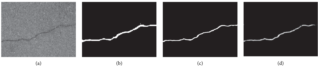
FIGURE 14: Transverse crack segmentation model results: (a) original image; (b) before improvement; (c) improved result; (d) ground truth.
