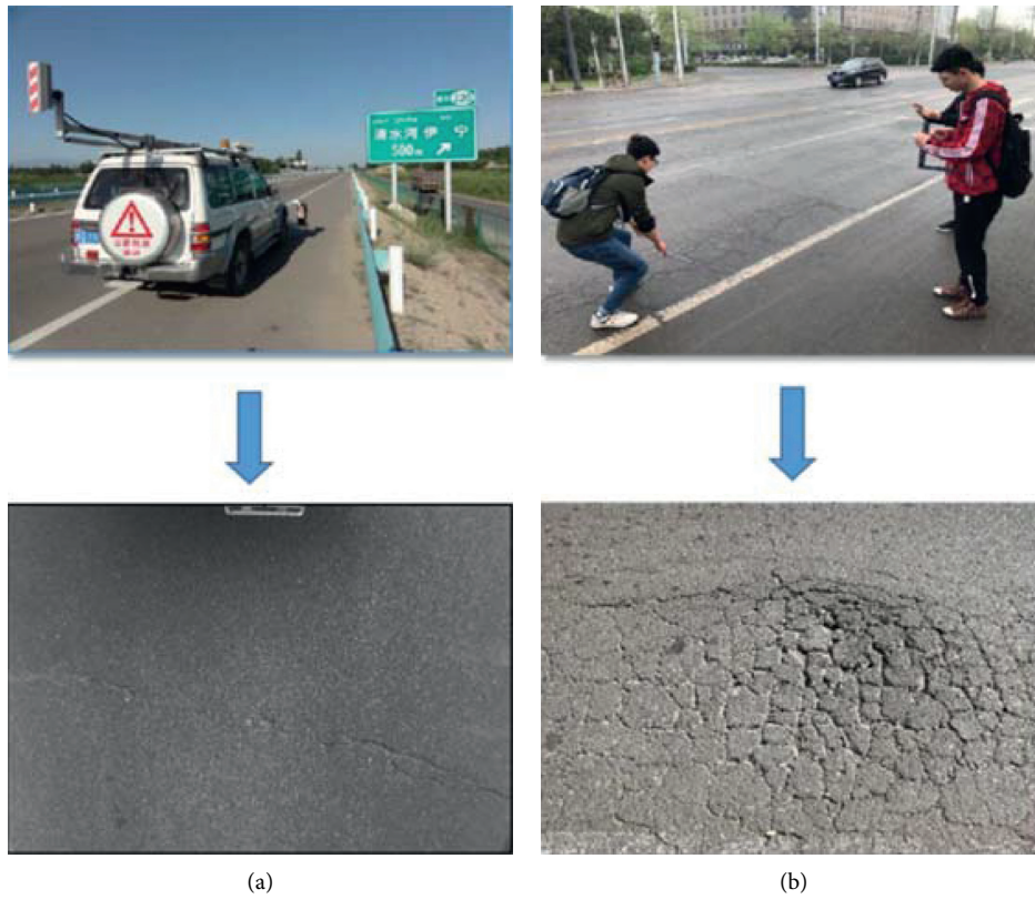
FIGURE 2: Pavement crack image acquisition and collection by (a) detector vehicle and (b) smartphone.
