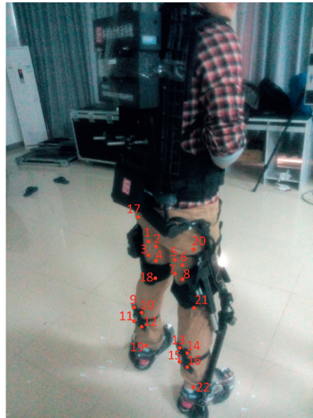
FIGURE 2: Diagrammatic sketch of the marker points and their locations: left/right thigh (marker no. 1–4/no. 5–8), left/right crus (marker no. 9–12/no. 13–16), left/right hip (marker no. 17/no. 20), left/right knee (marker no. 18/no. 21), and left/right ankle (marker no. 19/no. 22). Note that markers on the thigh are in front of them. So, they are invisible from this visual angle.
