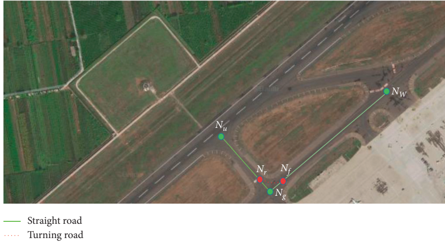
FIGURE 2: Aircraft turning section taxiing process.
