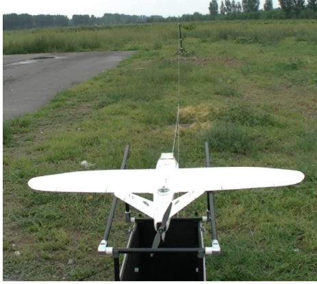
FIGURE 5: SUAV and ejection device.
