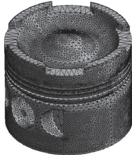
FIGURE 6: Meshing model of the piston.
