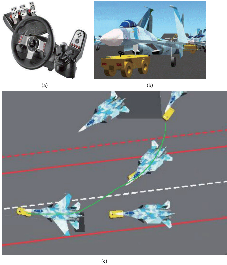
FIGURE 9: The carrier deck operation simulator environment. (a) The Logitech driving input device. (b) The simulated 3D tractor towing aircraft. (c) The tractor-aircraft movement and path generated (green line).
