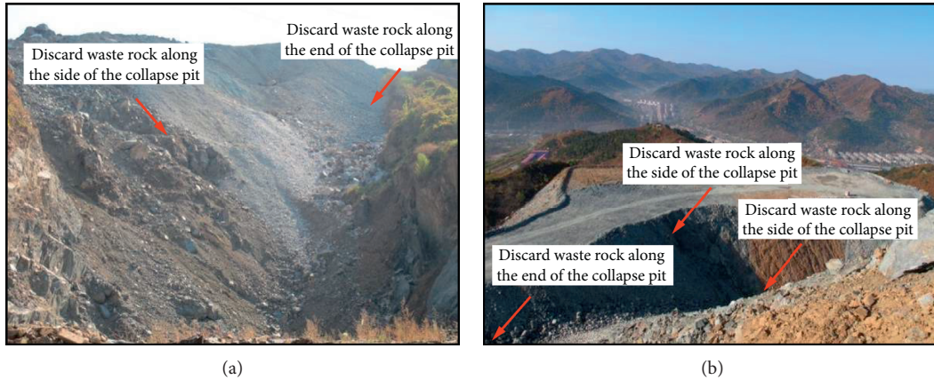
FIGURE 8: Collapse pit waste rock plan and site map. (a) Left view; (b) Top view.
