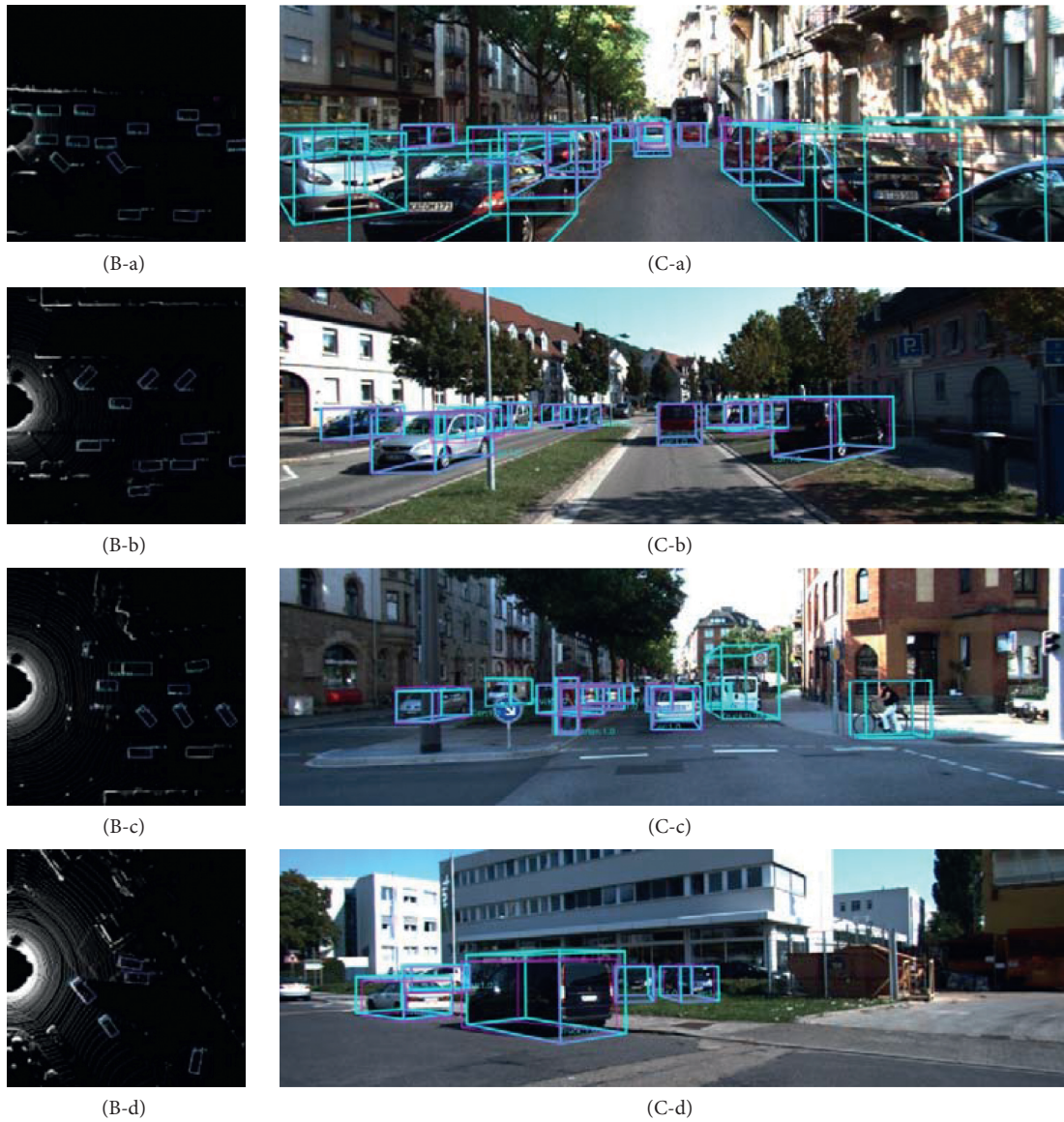
FIGURE 10: Recognition visualization of the KITTI dataset. (B, C) The bird's eye view and corresponding camera view separately; (a, b) multiobject scenes; (c) multicategory scene; (d) unordered objects scene.
