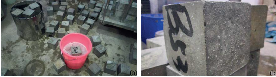
FIGURE 1: Inorganic coating spraying of concrete. (a) Concrete samples and coating material; (b) concrete surface morphology after inorganic coating spraying.
