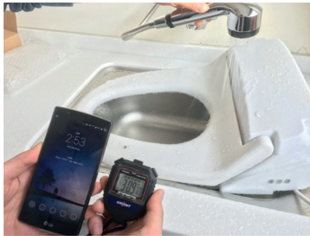
FIGURE 13: Experiment conducted to verify the waterproof capability of the smart health-monitoring bidet system.
