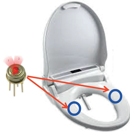
FIGURE 5: Smart health-monitoring bidet cover with the thermometer sensor.
