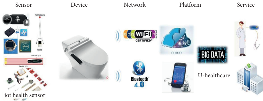
FIGURE 1: Smart health-monitoring bidet end-to-end architecture.
