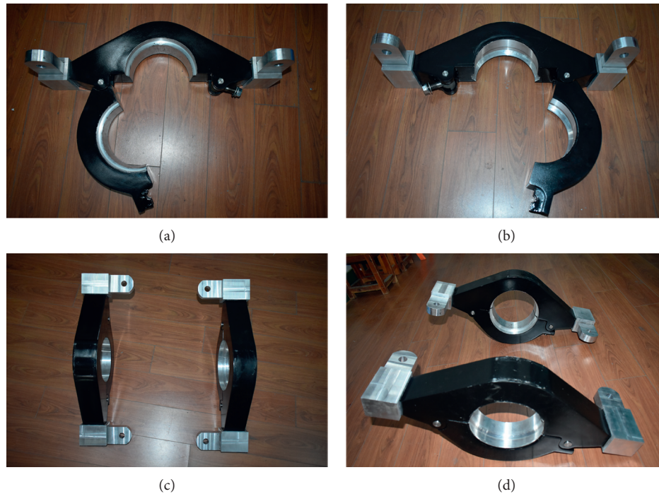
FIGURE 19: Carbon fiber closed clamp after test: (a) carbon fiber front fixture, (b) carbon fiber rear fixture, (c) overall top view of the carbon fiber fixture, and (d) overall side view of the carbon fiber fixture.
