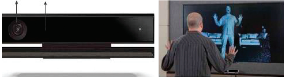
FIGURE 1: The appearance and structure of the second-generation Kinect and an example of obtaining depth images (the picture comes from https://image.baidu.com/ ).
