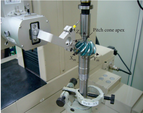
FIGURE 1: Schematic diagram of measuring coordinate system of spiral bevel gear.
