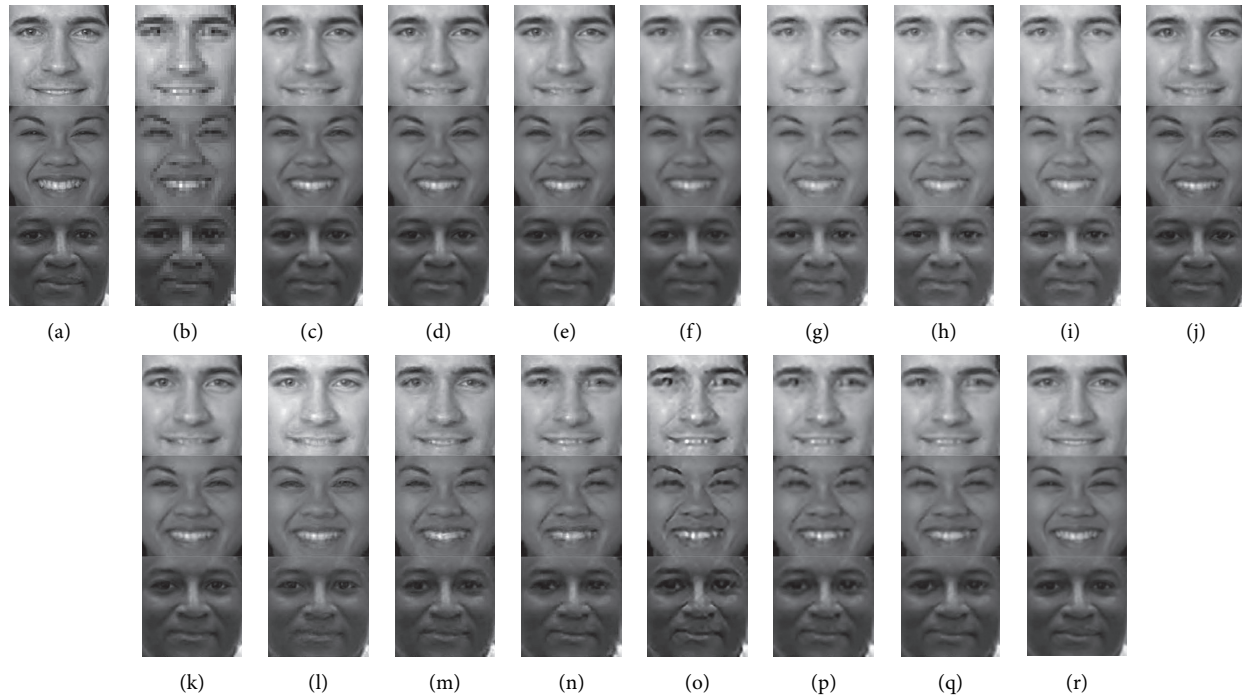
FIGURE 7: Comparison of face image super-resolution methods' results on FERET by different methods. (a) Original HR images. (b) LR input images. (c) LcR [13]. (d) SSR [41]. (e) LLT [12]. (f) Wang's [40]. (g) NE [14]. (h) SR [10]. (i) WSR [34]. (j) CDA [39]. (k) Bicubic [35]. (l) MSR [11]. (m) Yang's [10]. (n) Glanser's [36]. (o) DPSR [37]. (p) SRCNN [16]. (q) SRAHF [38]. (r) Ours.
