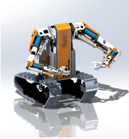
FIGURE 1: Modeling diagram of the humanoid 7-DOF hydraulically driven dual-arm robot.
