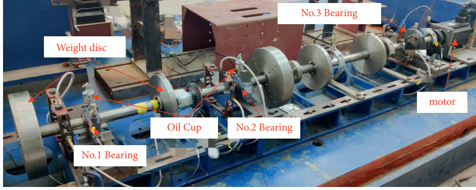
FIGURE 1: Actual structure diagram of the test rig.
