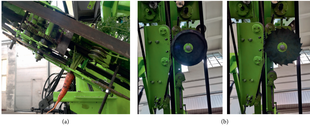
FIGURE 10: Bench test. (a) Cutting status. (b) Comparison between conventional tool and bionic tool.
