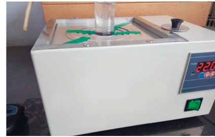
FIGURE 2: The control device of the water temperatures to observe the degassing processes of radon measurements.
