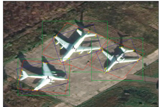
FIGURE 14: RANGE-MBR allows to build quasi-minimum bounding rectangles.
