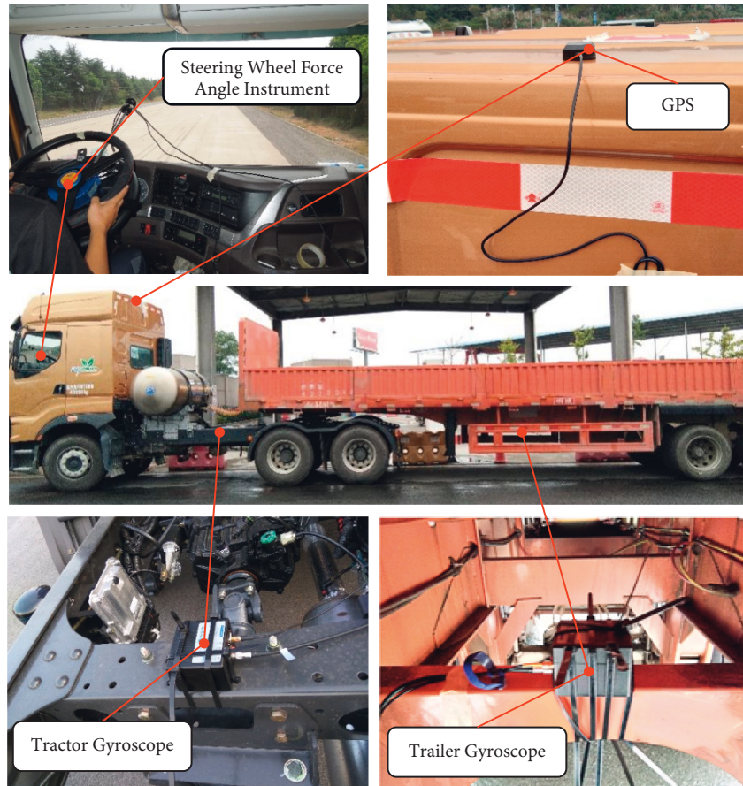
FIGURE 4: The installation position of test equipment.
