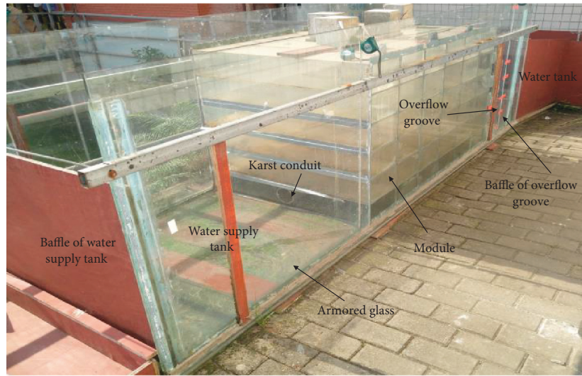
FIGURE 2: Physical diagram of the test model.
