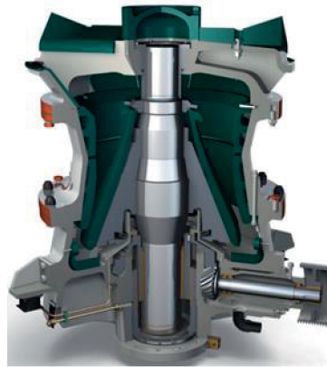
FIGURE 1: Structure diagram of cone crusher.
