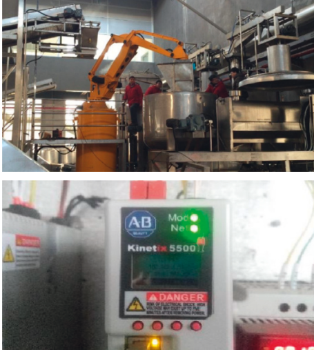
FIGURE 8: Part of the scene diagram of the automatic retort distillation production line and the robot motor driver.
