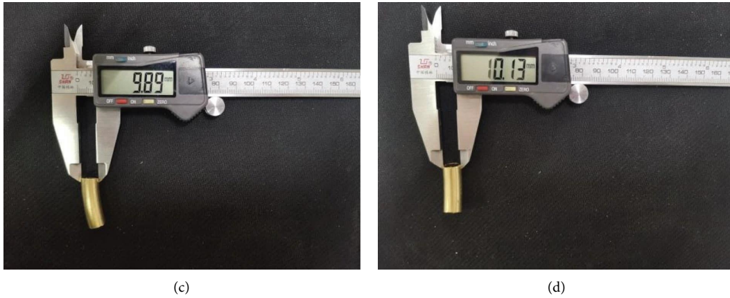
FIGURE 19: Wall thickness change and section distortion. (a) Inner wall thickness. (b) Outer wall thickness. (c) Minimum tube diameter. (d) Maximum tube diameter.
