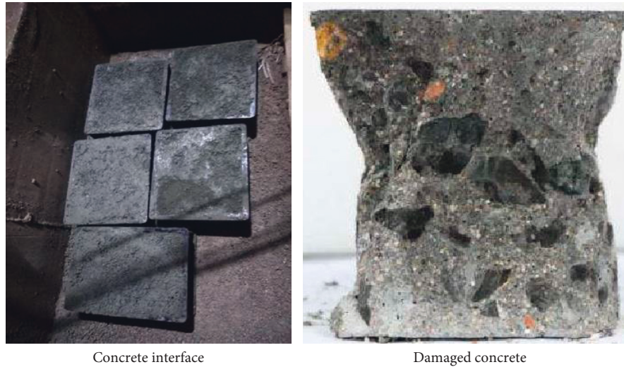
FIGURE 1: The concrete surface and the damaged concrete.
