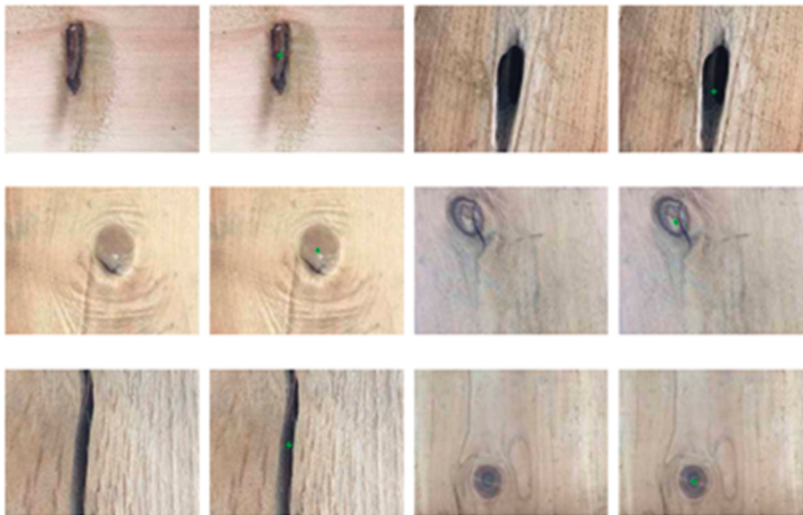
FIGURE 5: Location results of different wood defects.
